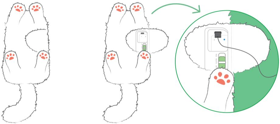
Open the pocket under metacat's belly, you will see the charging port and the three stages switch of metacat.
